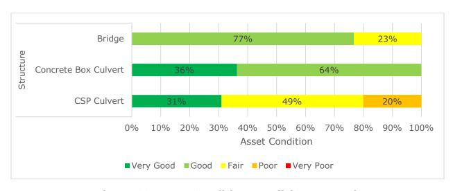
Figure 23: Asset Condition Detail (Structures)
