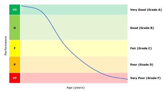
Figure 9: Schematic of an Asset's Deterioration Over Time
