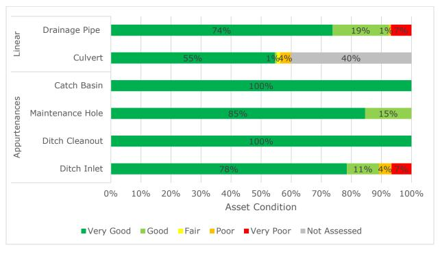
**Figure 27: Asset Condition Detail (Stormwater Management)**
