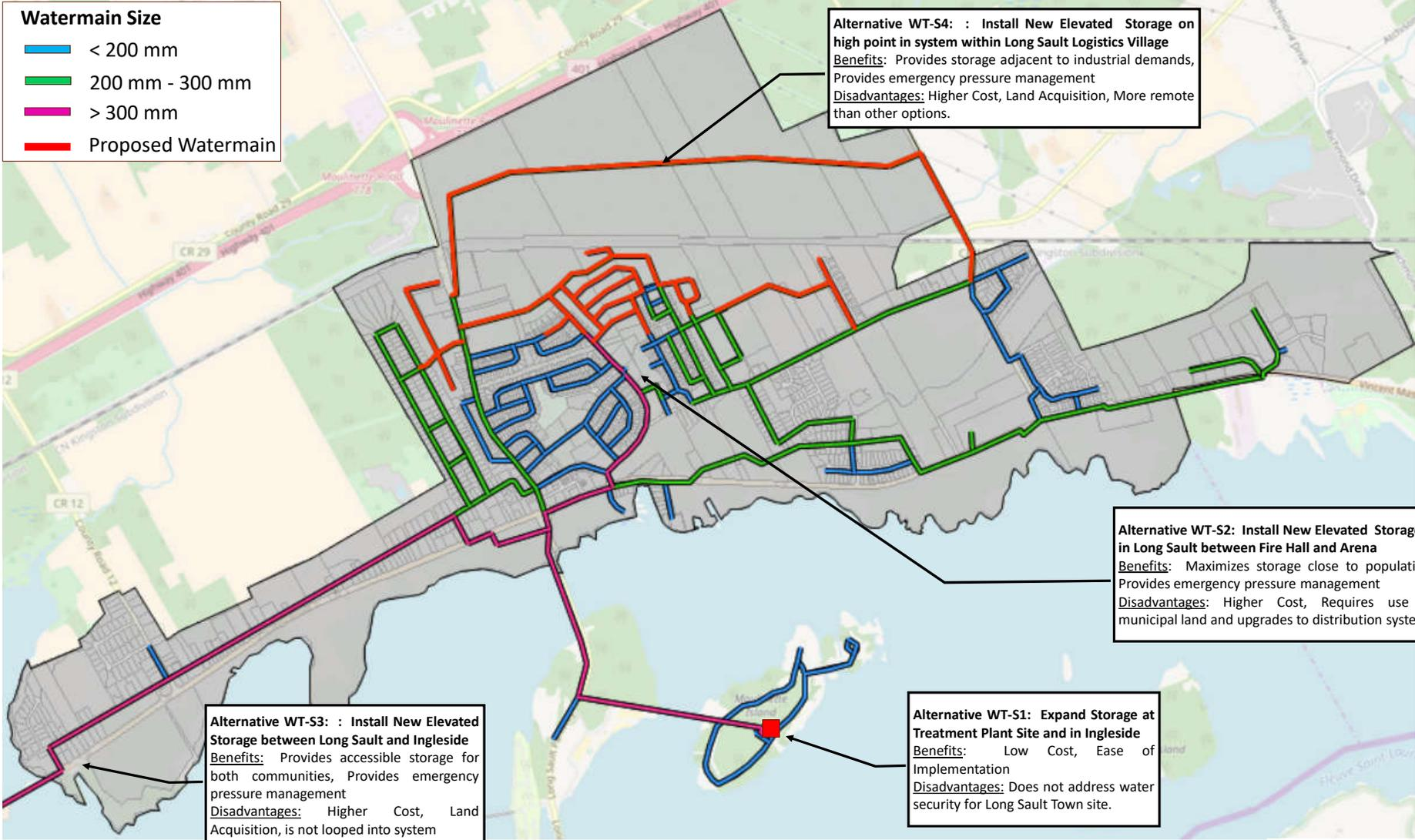
**Alternative WT-S4:** : Install New Elevated Storage on high point in system within Long Sault Logistics Village
