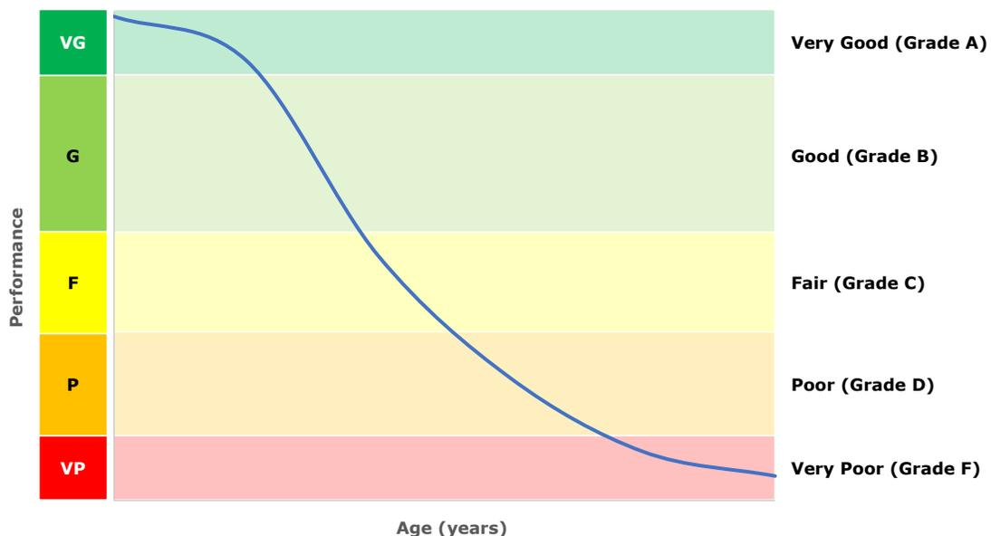
**Figure 9: Schematic of an Asset's Deterioration Over Time**
