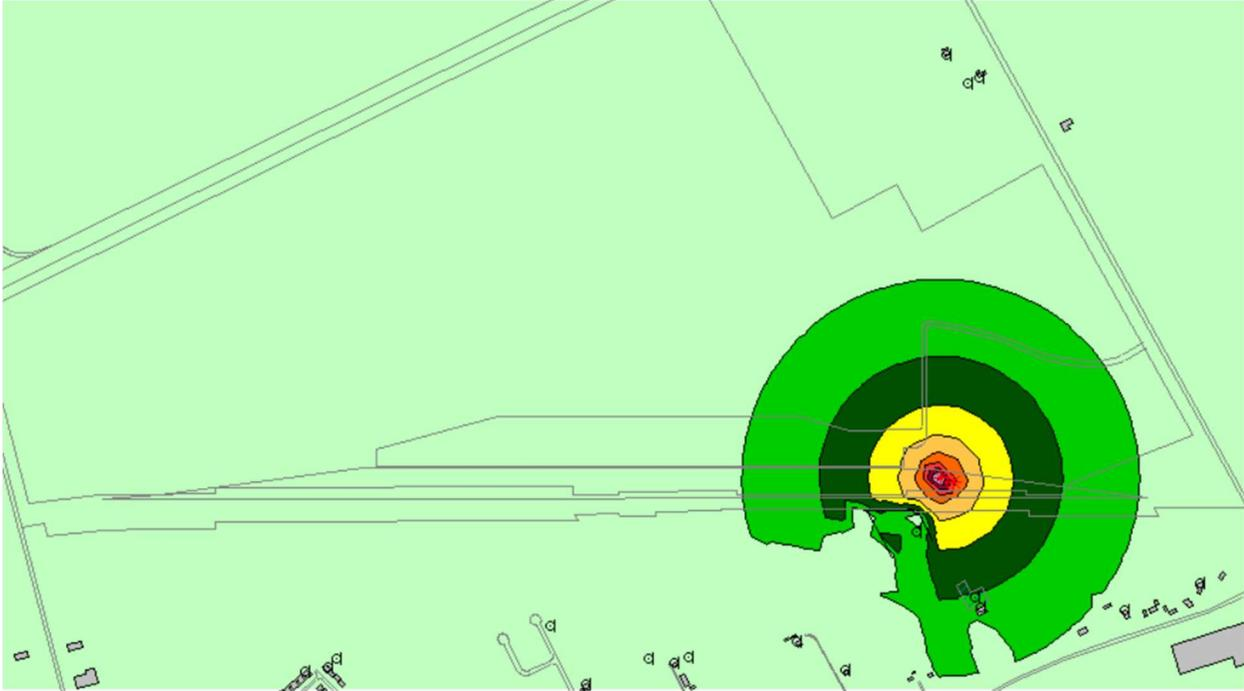
**FIGURE 4: EVENING AND NIGHTTIME STEADY-STATE / VARYING STATIONARY NOISE CONTOURS (1.5 METERS ABOVE GRADE)**
