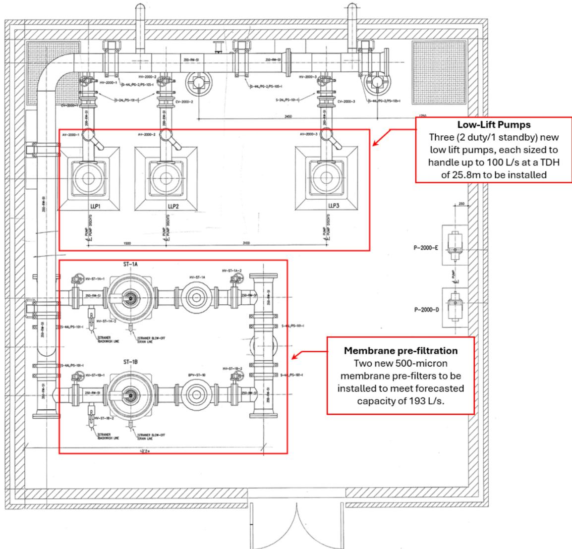
Figure 12-2 Low-Lift Station Upgrades
