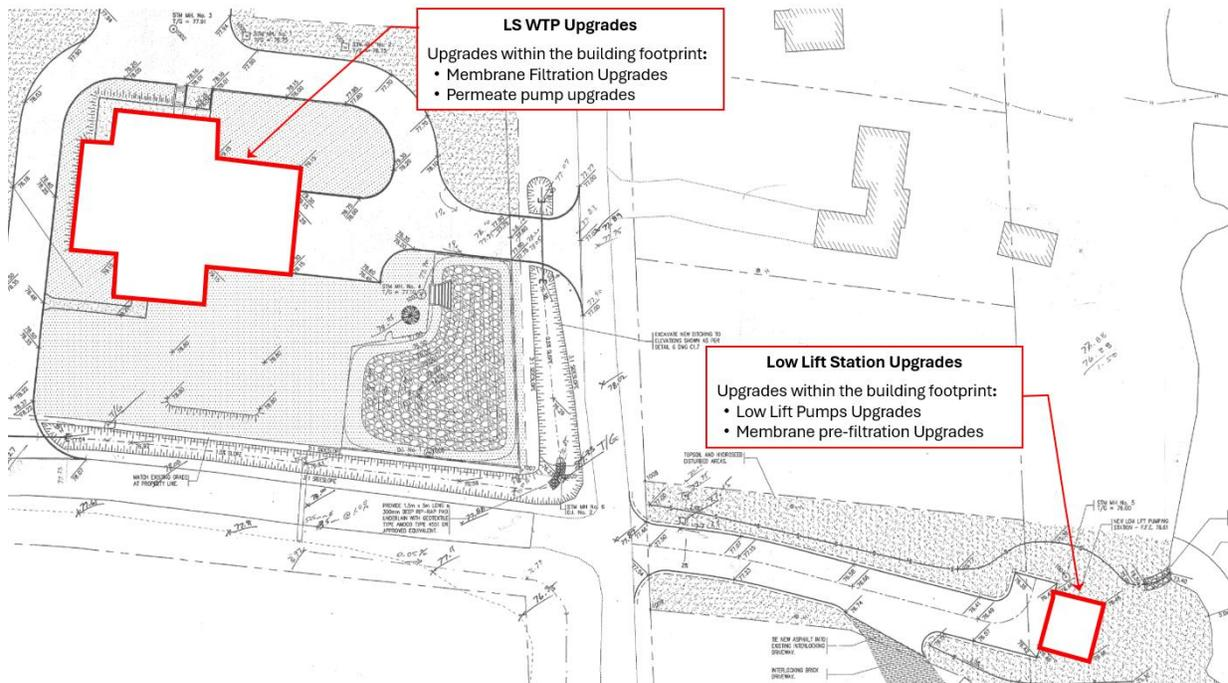
Figure 12-1 Long Sault WTP and Low lift station upgrades – Site Plan
